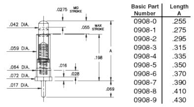
**Description:** 0908 - Spring-Loaded Pin Packaging: Packaged in Bulk
